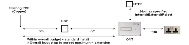
Telephony wiring back to NTE5 – an End User can choose internal or external (where practicable):
