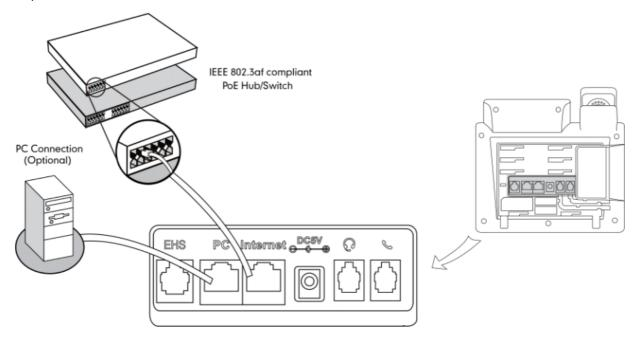
Note: If in-line power switch/hub is provided, you don't need to connect the phone to the power adapter. Make sure the switch/hub is PoE-compliant. The phone can also share the network with another network device
